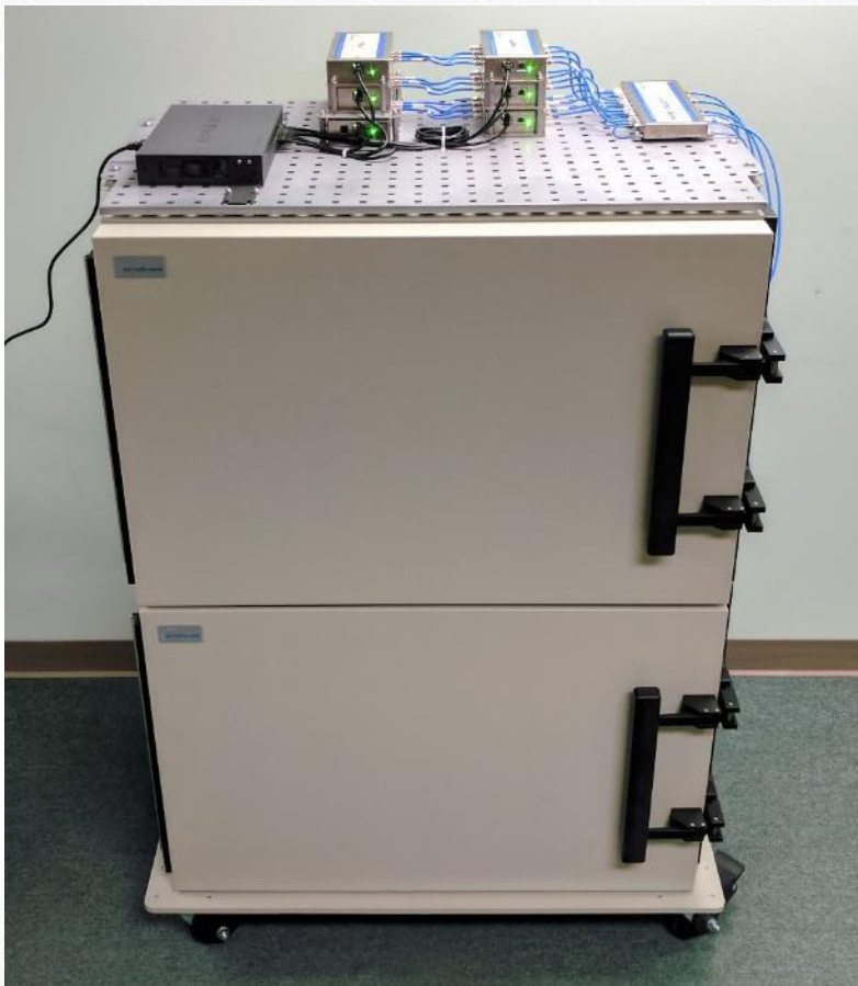
Stand-alone isolated testbed fits into a 40"W x 31"D footprint
